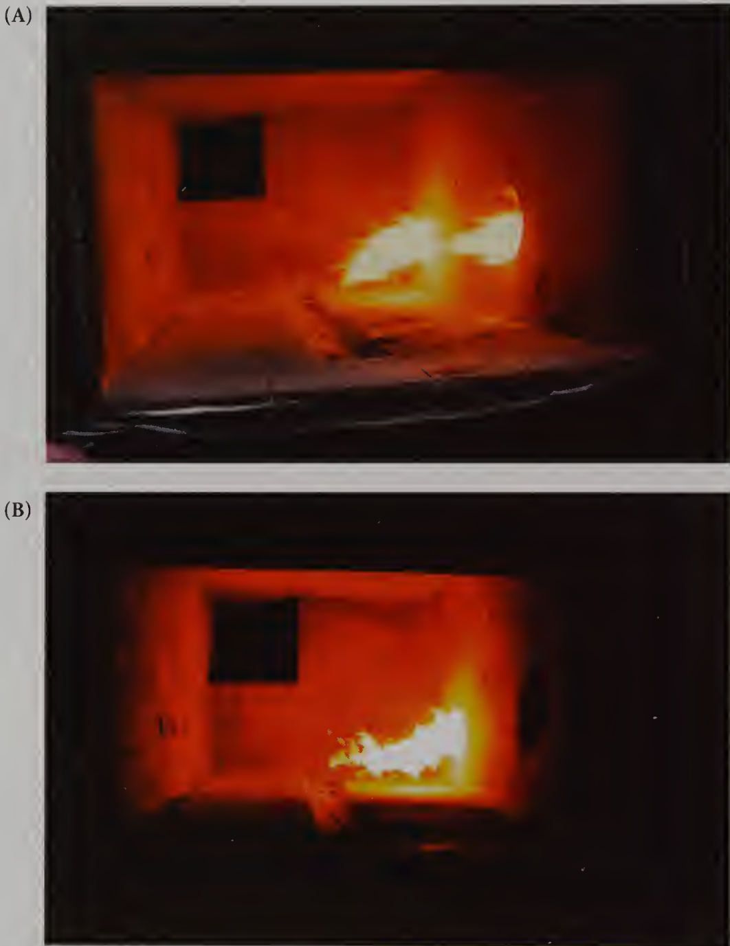
Figure 16.22 CREMATORIUM. Interior view of the crematorium used to cremate the victim alive. (A) The crematorium operating in a normal fashion. (B) The malfunctioning of the crematorium. Note that only one burner is operating. The killer was unaware of the second burner's malfunction. (Courtesy of retired Major John Dotson, Wichita, Kansas, Police Department and now chief in Sparks, Nevada.)
