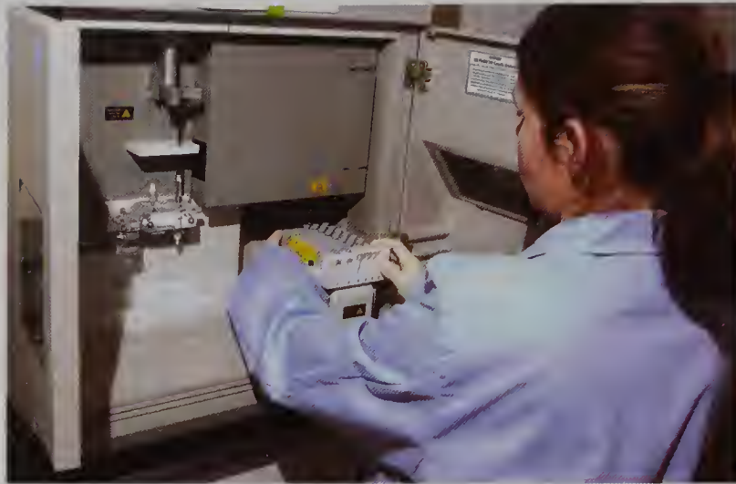
Figure 16.17 CAPILLILARY ELECTROPHERSIS UNIT. Forensic analyst Jennifer Reilly places samples in the ABI Pism 310 capillary electrophoresis (CE) unit. This instrument will analyze fragments of DNA to obtain a genetic profile. (Courtesy of Fred Drummond, chief of Forensic Sciences, Westchester County, New York, Forensic Laboratory. Photographer: Keith Mancini.)
