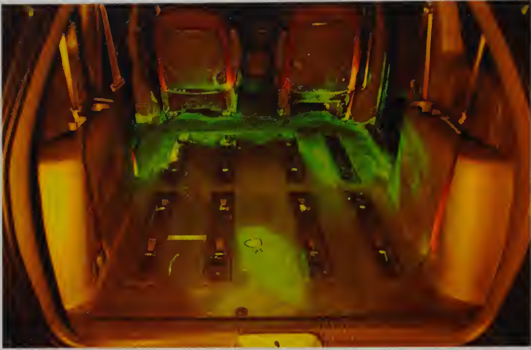
Figure 17.38 SUSPECT'S VEHICLE AFTER ALS. An alternate light source was used to view the interior of the van. Areas of the van fluoresced at 435 nm showing areas of possible cleaning with detergents. (Courtesy of Fred Drummond, chief of Forensic Sciences, Westchester County, New York, Forensic Laboratory. Photographs courtesy of Kevin MacLaren. Photographer: Keith A. Mancini.)
