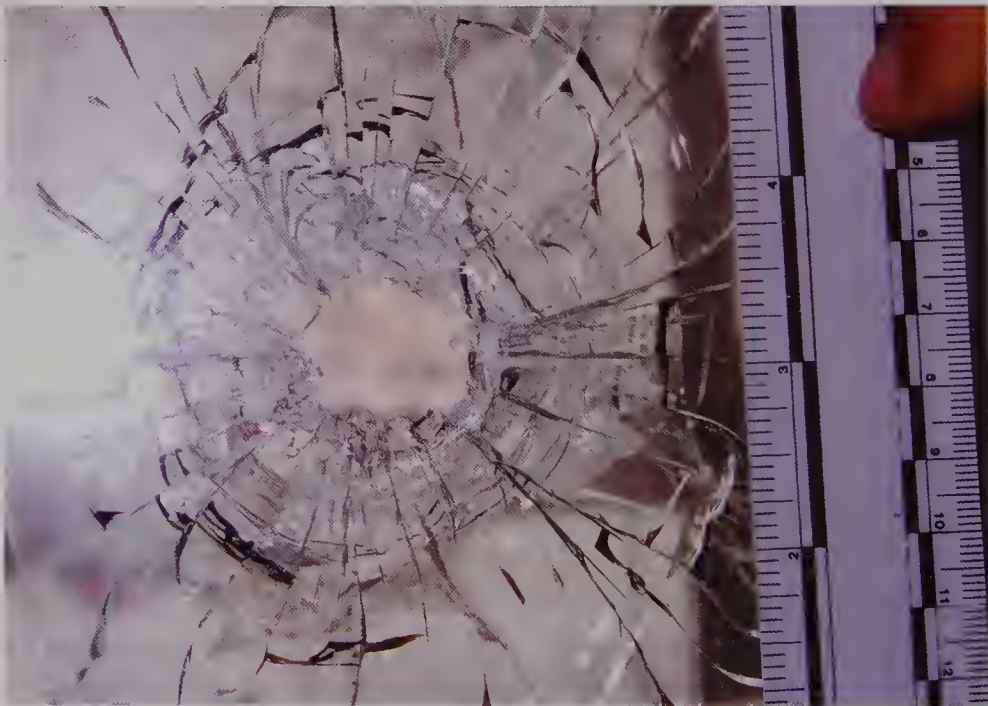
Figure 17.39 INSIDE WINDOW — SHOTS FIRED THROUGH GLASS. Multiple homicide scene. Witnesses described two offenders who began shooting through the open doorway of a crowded night club. Evidence collected inside the club indicated that shots had also been fired from inside the club toward the first two shooters. Everyone inside the club denied that shots had been fired from inside. Bullet holes were discovered in the plate glass windows at the front of the club. The inside window depicted in this photograph has a nearly symmetrical hole in the glass. (Courtesy of Detective Mark Czworaniak, Chicago Police Department.)
