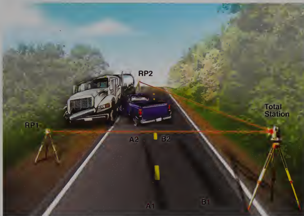
Figure 7.12 TOTAL STATION CALCULATES THREE-DIMENSIONAL COORDINATES. The drawing here represents the sophisticated Total Station system's ability to take crime scene measurements. (Courtesy of Medical Legal Art. Illustration copyright 2005, Medical Legal Art, www.doereport.com .)
