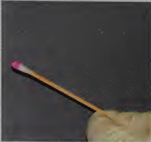
Figure 17.5A PHENOLPATHLEIN. Phenolphthalein is a presumptive blood test. The swab is moistened with dionized water. Swab the area of interest with the dampened swab. Add one or two drops of phenolphthalein. Then add one or two drops of hydrogen peroxide. If blood is present, the swab will turn a purple/fuchsia color immediately. (Courtesy of David Rossi, CSI/SCSA, Harris County, Texas, Sheriff's Department.)
