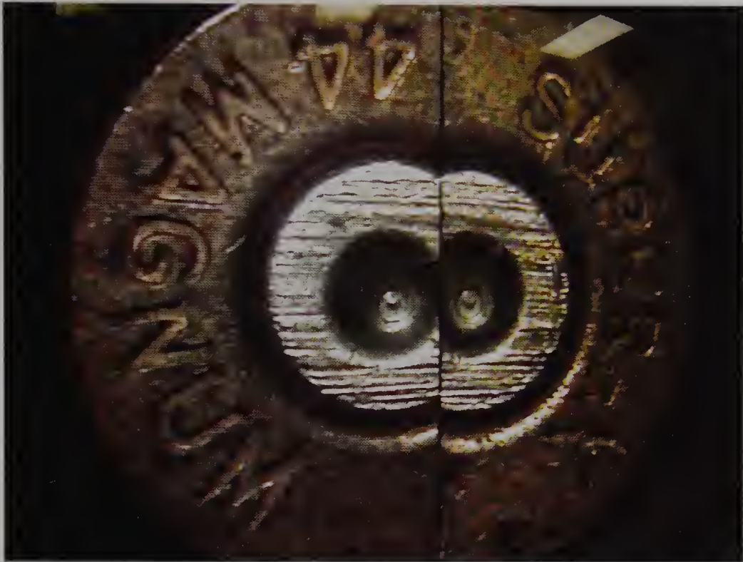
Figure 17.23 POSITIVE COMPARISON — CARTRIDGE CASE. Positive comparison of two .44 magnum caliber discharged cartridge cases. The individual characteristics of each discharged cartridge case consist of horizontal breech face markings and a unique firing pin indent. (Courtesy of Detective Sergeant Frank Nicolosi and Detective Sergeant Anthony Tota, Westchester County, New York, Police Department's Ballistics Unit.)
