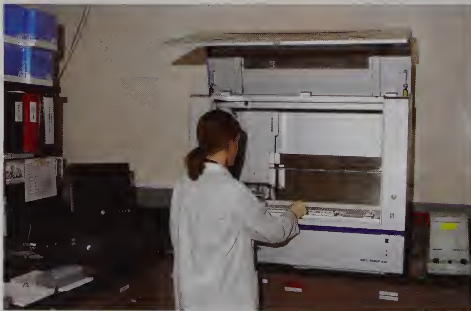
Figure 16.10 THE QIAGEN M48 BIOROBOT. The Qiagen M48 BioRobot is designed to make the extraction of DNA samples less time consuming. The robot automatically transfers reagents and samples from tube to tube using magnetic beads to hold the DNA and allow its purification. (Courtesy of Fred Drummond, chief of Forensic Sciences, Westchester County, New York, Forensic Laboratory. Photographer: Keith Mancini.)
