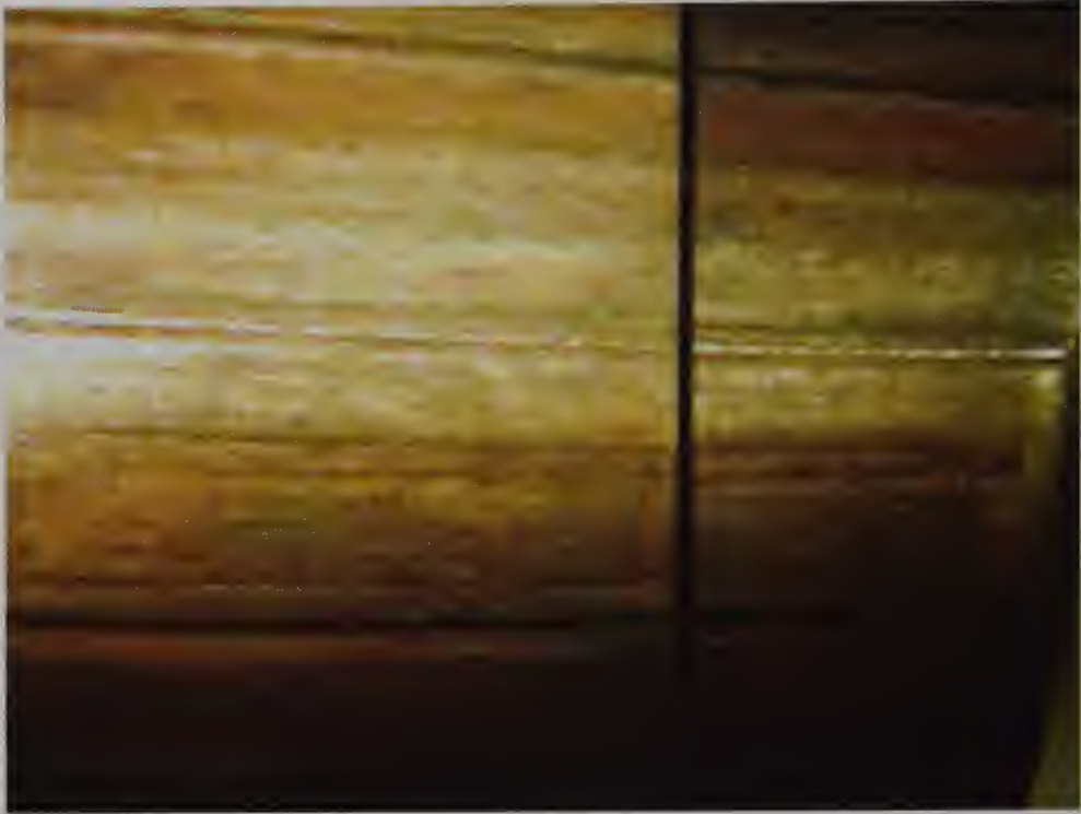
Figure 17.24 POSITIVE COMPARISON — BULLETS. Positive comparison of two .45 caliber copper-jacketed bullets. The individual characteristics on each bullet include striations that appear on the land and groove areas. The striae that appear on these bullets are accidental in nature and unique to a particular firearm. (Courtesy of Detective Sergeant Frank Nicolosi and Detective Sergeant Anthony Tota, Westchester County, New York, Police Department's Ballistics Unit.)
