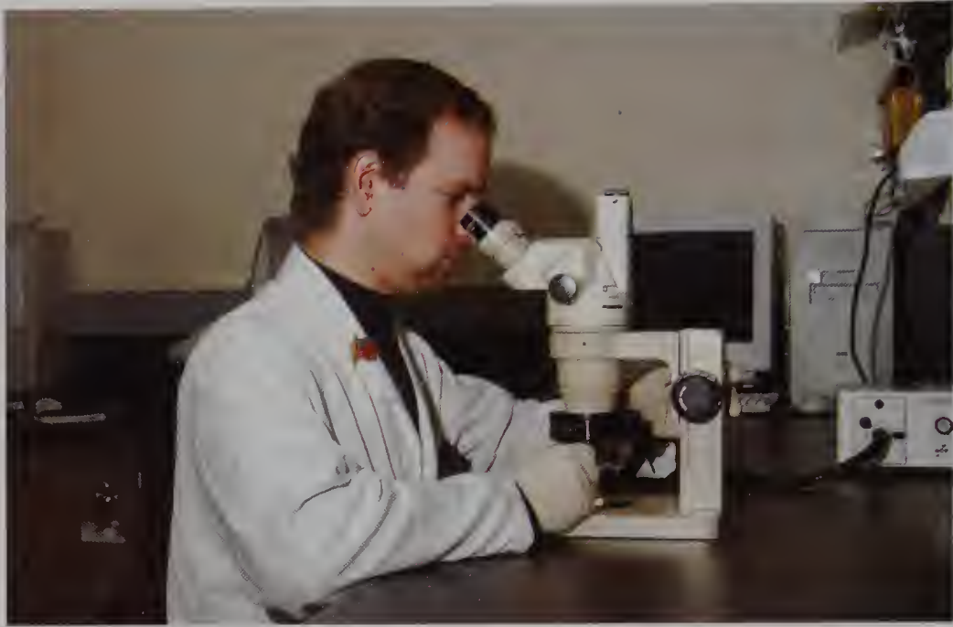
Figure 17.32 EXAMINATION FOR TRACE EVIDENCE. Forensic scientist Daniel Rothenberg examines trace evidence under a stereomicroscope, which provided a three-dimensional image. (Courtesy of Fred Drummond, chief of Forensic Sciences, Westchester County, New York, Forensic Laboratory. Photographer: Keith Mancini.)
